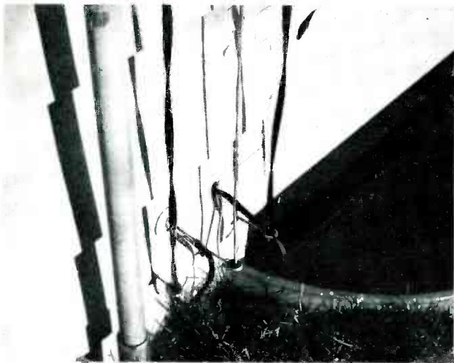
Fig. 10 Eyelet-type standoff shown here acts as a shorted turn around UHF lead-in, causing multiple ghosts and other similar trouble symptoms on the TV screen.
