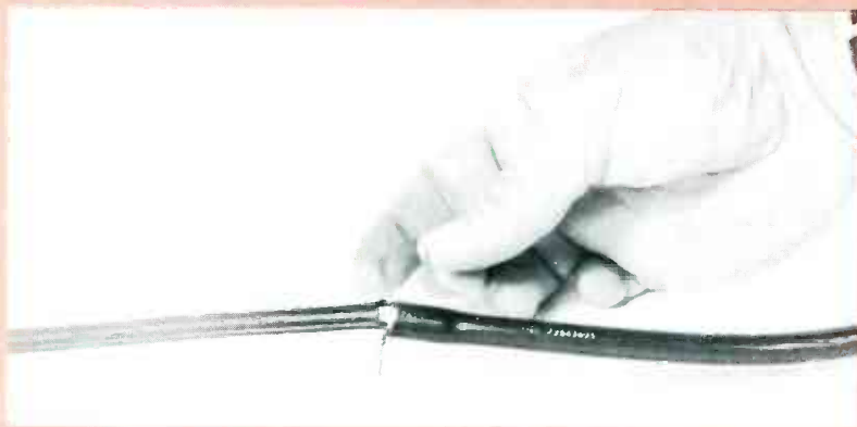
(C) Twist wires securely.
