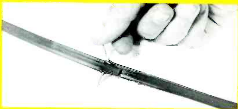
(B) Overlap tabs and twist wires
